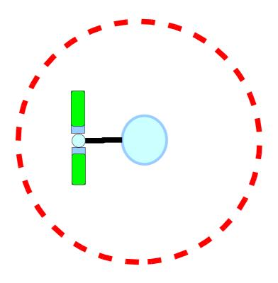
In the above diagram: Red denote Magnets, all the Magnet has poles facing inward. Deep Blue denote metallic core. Light Green denote generating coil.
