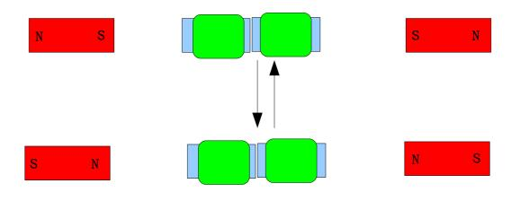
2. Another method to neutralize drag force: First the drag force produce a clockwise torque, then the drag force produce an anti-clockwise torque. Two torques are acting in the same system to neutralize the effect of each other.
